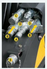
A connect under pressure CUP hydraulic manifold is standard equipment on all models for easy hook-up of all hydraulic attachments. By pushing on the fitting, you release pressure in both hydraulic lines.
